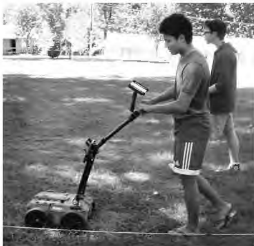
FIGURE 8. Student participants operating the ground-penetrating radar in the Old College area. Thomas Alvarado '21 is pushing the GPR cart and Jonah Popp '21 is maintaining notes of the survey line. View is to the west.
