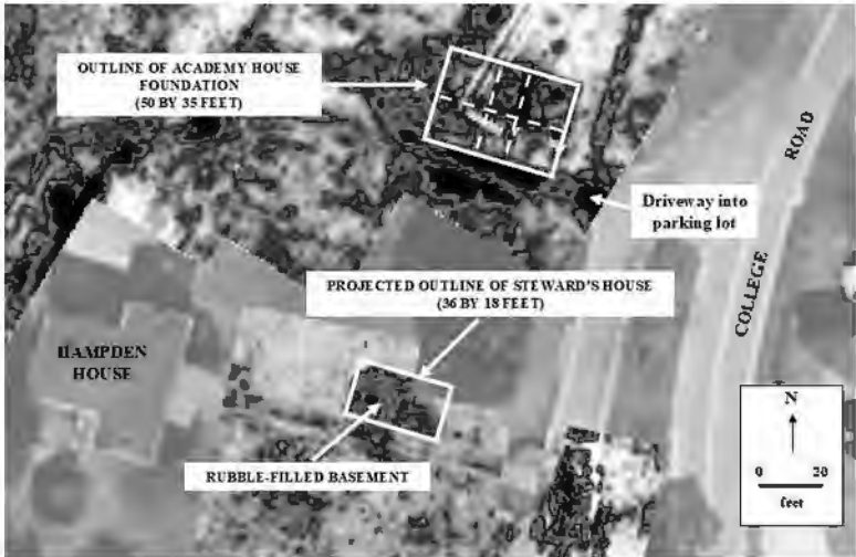
FIGURE 11. Ground-penetrating radar image of Academy House & Steward's House.
